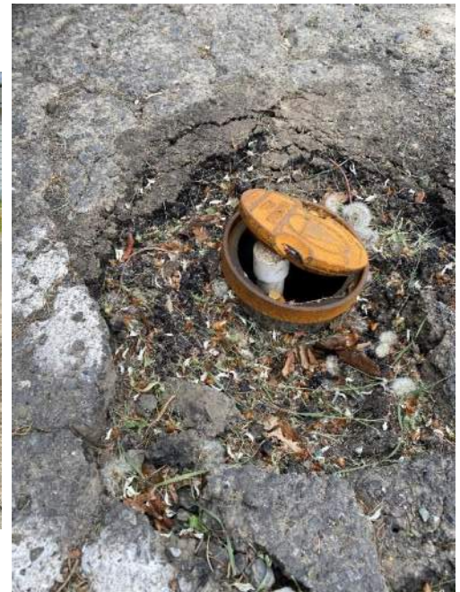
05/11/2021: BH-05 after completion as a piezometer with flush-mount monument (left). After approximately a month, ground had subsided around the monument and left the casing protruding above the lip of the monument (right). The casing was cut down so the monument lid could be closed.
