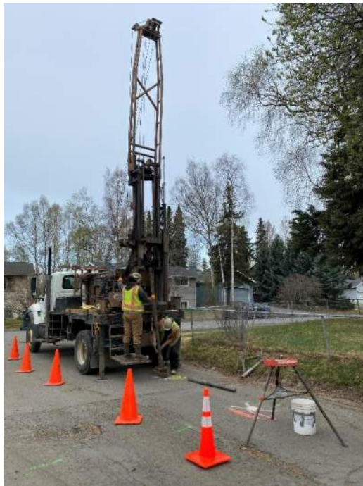
05/11/2021: Setting up rig on BH-03 with utility markings (left). Borehole marked with white paint. BH-03 after completion as a piezometer with flush-mount monument (right).
